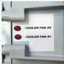
INDICATOR LEDS ON THE SIDE OF THE ENCLOSURE
